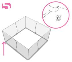
Place the graphic underneath the frame. Pull up the graphic and cover the entire frame. Make sure the printed graphic faces outwards and the prehemmed holes are aligned with the top screws. Insert the eyehooks along the pre-hemmed holes.
