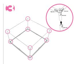
• Then connect the vertical straight tubes (Blue Colored Label: T & B) to the top and bottom corner connectors.
