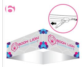
• Using the industrial-size-zipper, zip above the top tube, maximizing fabric tension. And zip to closed.
